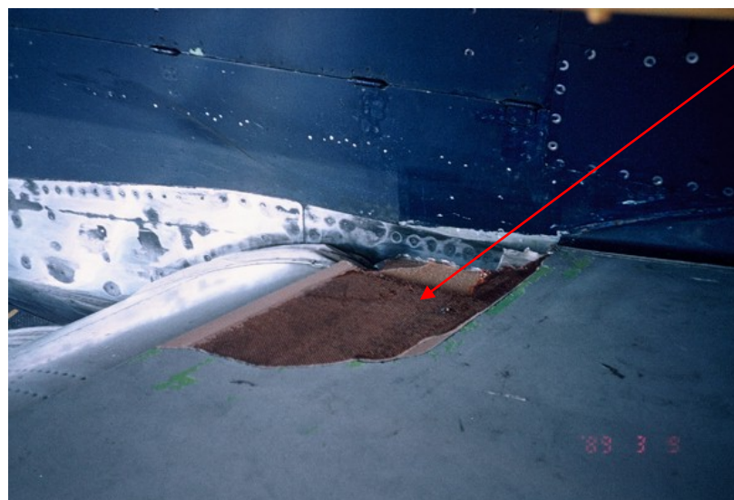
Inboard Flying Panel – partial separation (SB747-57-2261)
